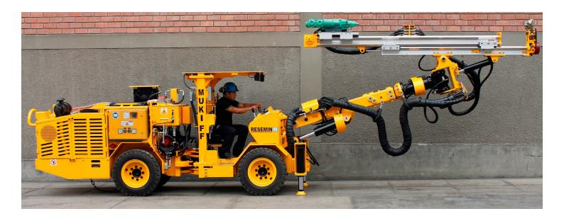
Front face drilling rig, electro-hydraulic, of 1.05 m width for tunneling in underground mining for small sections from  $1.5 \times 2.0$  up to  $3.5 \times 3.5$  m. Upper Drill option, for Cut & Fill method on sections from 1.5 m width at the bottom.
