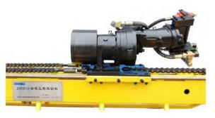
Different models have different rotation units. The spindle inner diameter is 58 mm. To replace the clamp in the chuck can help hold drill rods of different diameters. With hydraulic motor, the spindle has infinitely variable speed. Drilling of low rotational speed and large torque can come true if the gear box be replaced with a pair of gears of 1:2.5 transmission ratio.
